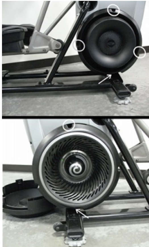
The top image is the lower right fan cover. The white arrow indicates the location of the power plug wire inlet and bottom screw, which can be loosened 3 turns rather than removing it entirely. The white circles indicate the locations of the screws to remove for removing the cover. The bottom image indicates the locations of the screws for the lower left fan cover.
