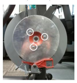
The three screws (circled in white) need to be removed so that the brake disc can be removed for troubleshooting.
