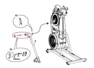
The red oval shows the cap and bolt to remove before removing the pedal arm from the crank.
