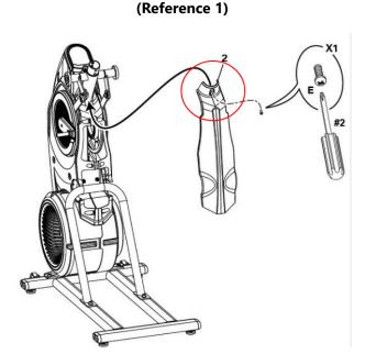
The red circle indicates the location of the screw to remove on the rear shroud.
