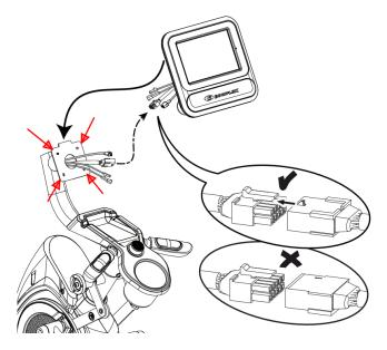
Disconnect all 4 cables and only reconnect the cable with 2 rows of 7 pins.
