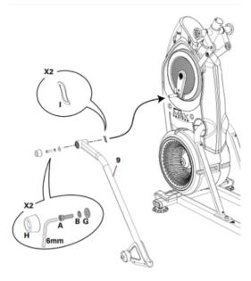
The Wave Washers (part labeled 'I') should be installed on the crank arm, indicated by the black arrow.
