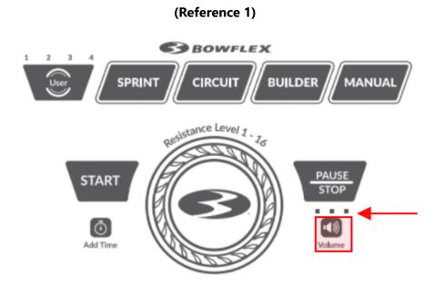
The volume button is shown in the red square. The red arrow points to the lights that should be illuminated when the sound is turned up.
