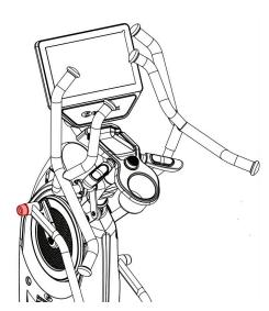
The end cap (highlighted red) is the small rubber component located at the pedal arm and crank arm connection.
