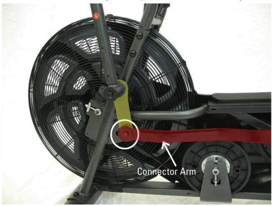
The arm pivot is highlighted in yellow and the connector arm is highlighted in red.
