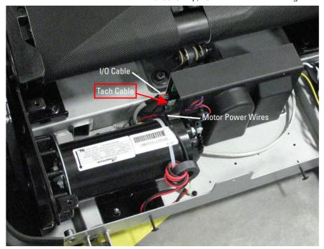
Inspect the bundle of wires for damage and make sure that the wires are firmly connected at the MCB.
