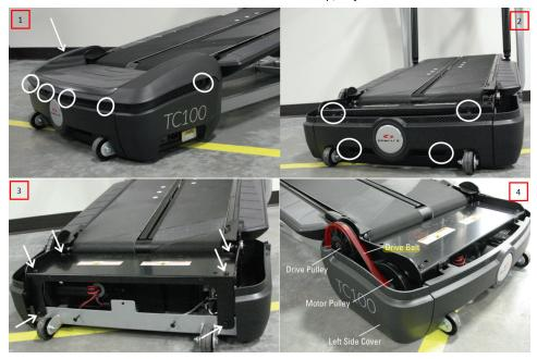
Remove the 6 screws on the rear step (1) and set the step to the side. Remove the 2 upper screws and loosen the 2 lower screws on the rear cover (2), then lift and slide the cover off. Remove the 6 bolts on the motor compartment cover and set the cover to the side (3). Inspect the drive belt (highlighted red) (4).
