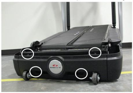
Remove the upper screws circled and loosen the lower screws, then lift and slide the rear cover off of your machine.
