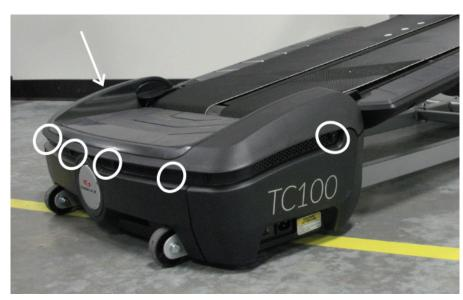
Remove the screws indicated on the rear step and set the rear step to the side.
