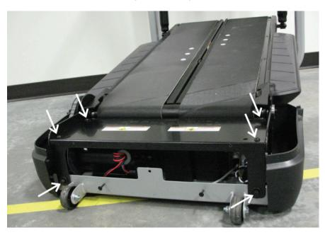
Remove the 6 bolts indicated on the motor compartment cover, then remove the cover and set it off to the side.
