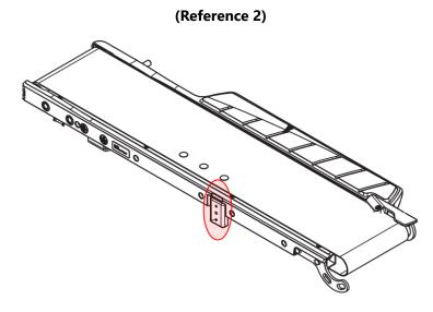
The friction block is circled in red - inspect for damage and check if it is loose or wobbly.
