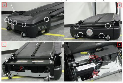
Remove the 6 screws on the rear step (1) and set the step to the side. Remove the 2 upper screws and loosen the 2 lower screws on the rear cover (2), then lift and slide the cover off. Remove the 6 bolts on the motor compartment cover and set the cover to the side (3). Inspect the I/O Cable indicated (4).
