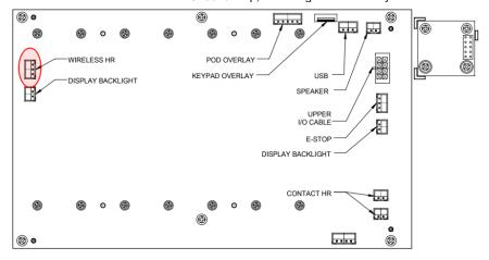
Inspect the wire and connection at the WIRELESS HR connector on the circuit board (circled in red).
