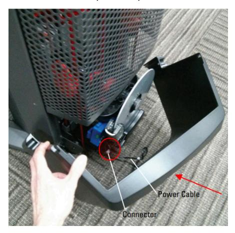
The power cable must be unplugged from the power inlet plug before continuing with removing the cover.
