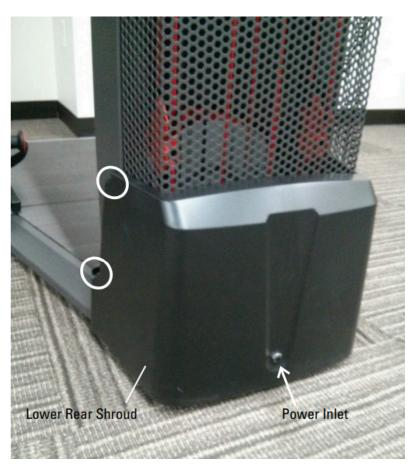
2 of the 4 screws to remove are circled. The other 2 screws are located in the same location on the opposite side of the shroud.
