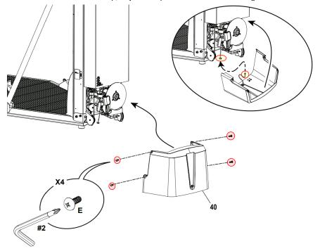
The screws to remove are circled in red. Unplug the power inlet wire (red/yellow circles) before completely removing the rear cove
