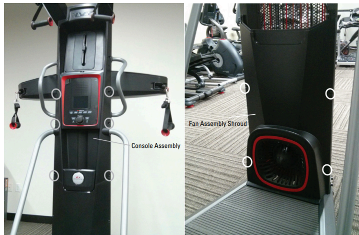
Remove the 10 screws from the shrouds. Remove the shrouds and set them to the side to inspect the ropes/pulleys.
