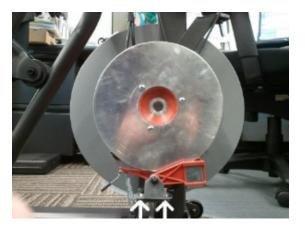
The white arrows indicate the location of the bolts to loosen in order to adjust the brake magnets.
