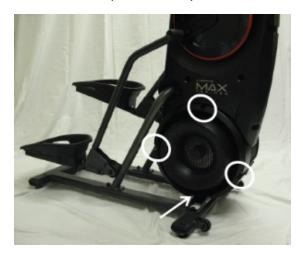
The white arrow indicates the location of the power plug wire inlet and bottom screw. The bottom screw can be loosened 3 turns rather than removing it entirely. The white circles indicate the locations of the screws to remove in order to remove the cover.
