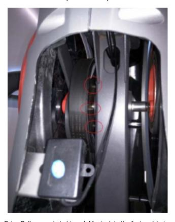
The screws attaching the Main Drive Pulley are circled in red. Manipulate the foot pedals to rotate the pulley and check all 4 screws, using a flashlight as necessary for better viewing.
