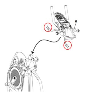
The bolts to remove are circled in red. Use a 5mm Allen wrench to remove and lift the console from the console mast.
