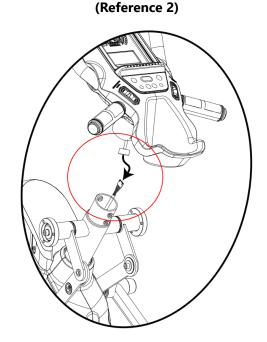
Check the cable connection circled in red. Unplug and firmly reconnect, paying special attention to the orientation of the connectors.
