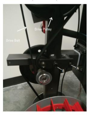
White arrows indicate the location of the drive belt and pulley.
