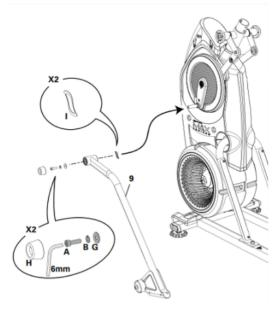
The Wave Washers (part labeled 'I') should be installed on the crank arm, indicated by the black arrow.
