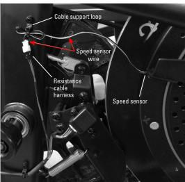
The speed sensor is located near the flywheel. Check the cable connection (red arrows) for damage and ensure it is firmly connected.
