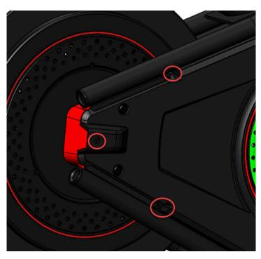
Remove the three screws from the right side of the flywheel, circled in red.
