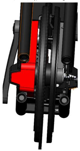
The shroud highlighted in red needs to be pulled back to access the flywheel and any potential glue/debris inside.
