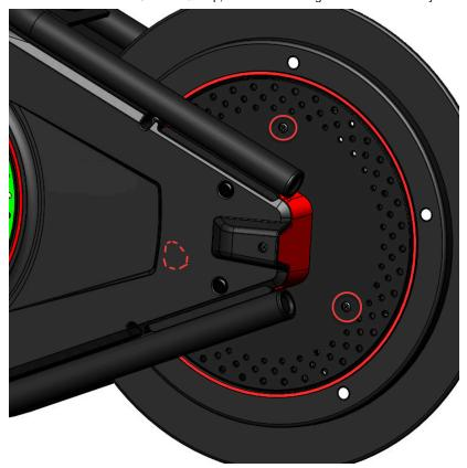
The three screws to remove from the left side of the flywheel are circled in red. Note that the third screw (on the left) can only be accessed by rotating the flywheel to expose the screw.
