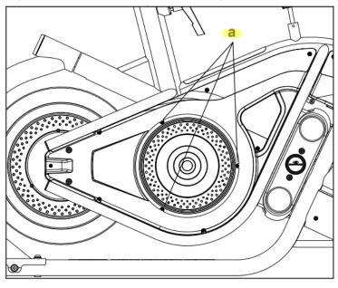
Starting with the bottom screw, remove the 3 screws (a) attaching the center disc to the shroud.
