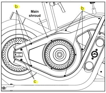
Starting with the bottom screws, remove the 9 remaining screws (b and c), then angle and remove the shroud.
