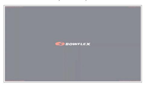
The initial screen showing the BowFlex or JRNY logo appears with serial numbers in each corner. Tap the upper right corner 10 times within 3 seconds to access the menu to force an update.
