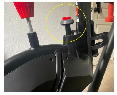
The cam is engaged by operating the tilt button, circled in yellow. Look inside the bike, directly below the tilt button, to see the cam.
