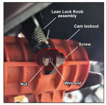
The lean lockout handle is connected to the lockout cam at the location circled in red.
