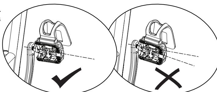
2. With the Pedal started by several hand turns into the Crank Arm, fully tighten it with the 15 mm Wrench.
