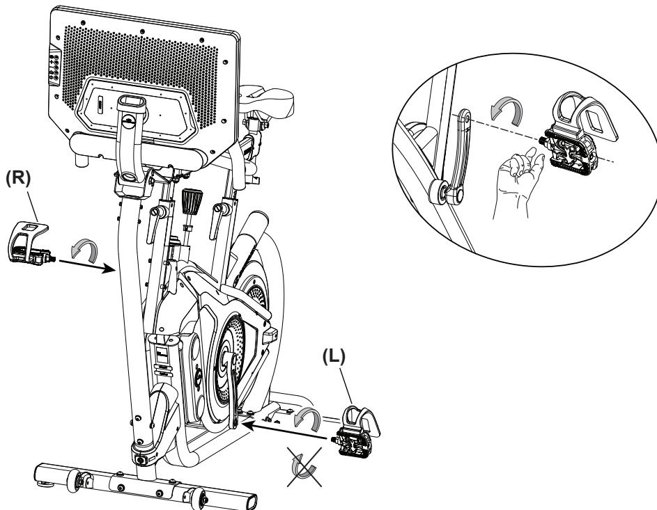
1. Start the Pedal by hand. If you feel resistance and the Pedal does not turn smoothly into the Crank Arm, make sure that the threads are aligned correctly. Be sure that the Pedal is going on straight into the Crank Arm. If the Pedal is not in-line with the opening, remove the Pedal and start again.
