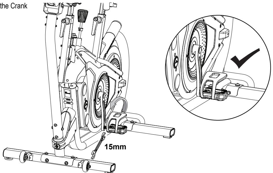
3. Confirm that the Pedal is fully tightened with the 15mm Wrench.
