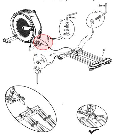
Inspect the rear stabilizer for grease (circled in red).
