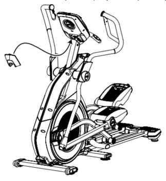
The shroud (pictured on the left) does not require any tools to remove. Pop it out of place to begin the console removal process.
