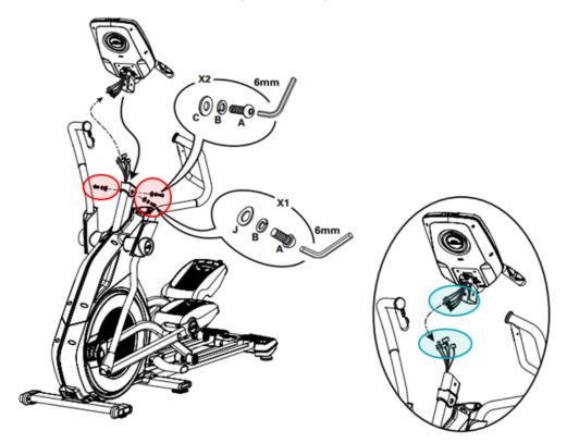
The bolts circled in red need to be removed to access the cables between the console and the console mast.
