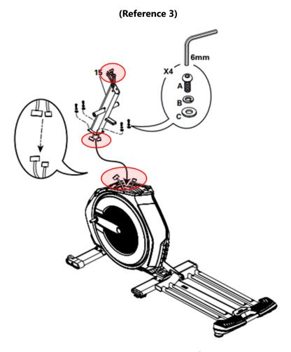
Inspect the 12-pin cables circled in red for damage.
