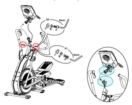
The bolts circled in red need to be removed to access the cables between the console and the console mast.
