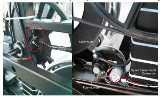
The speed sensor is circled in red on the left side. Inspect the speed sensor and wire (red arrow) for damage. Follow the wire back to the servo motor harness connection (circled in red on the right) and make sure it is securely connected.
