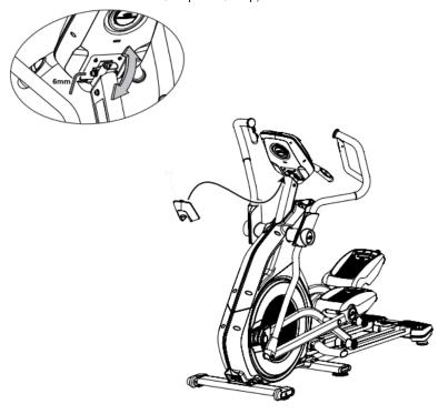
The shroud (pictured mid-image) does not require any tools to remove. Pop it out of place to begin the console removal process.
