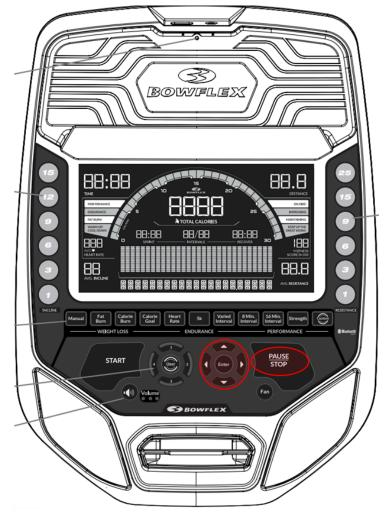
Press and hold the circled buttons for 3 seconds to exit Demonstration Mode.
