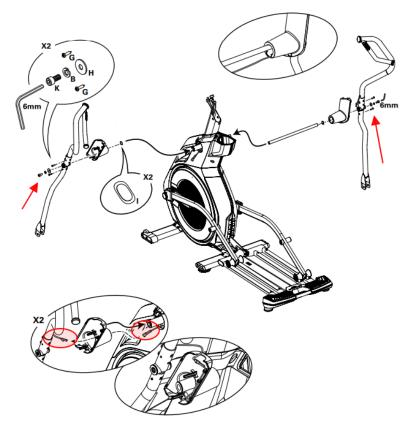
*Remove and disassemble the upper handlebars to inspect the wiring contained inside. The wiring is circled in red and the locations of the bolts are shown using the red arrows.*
