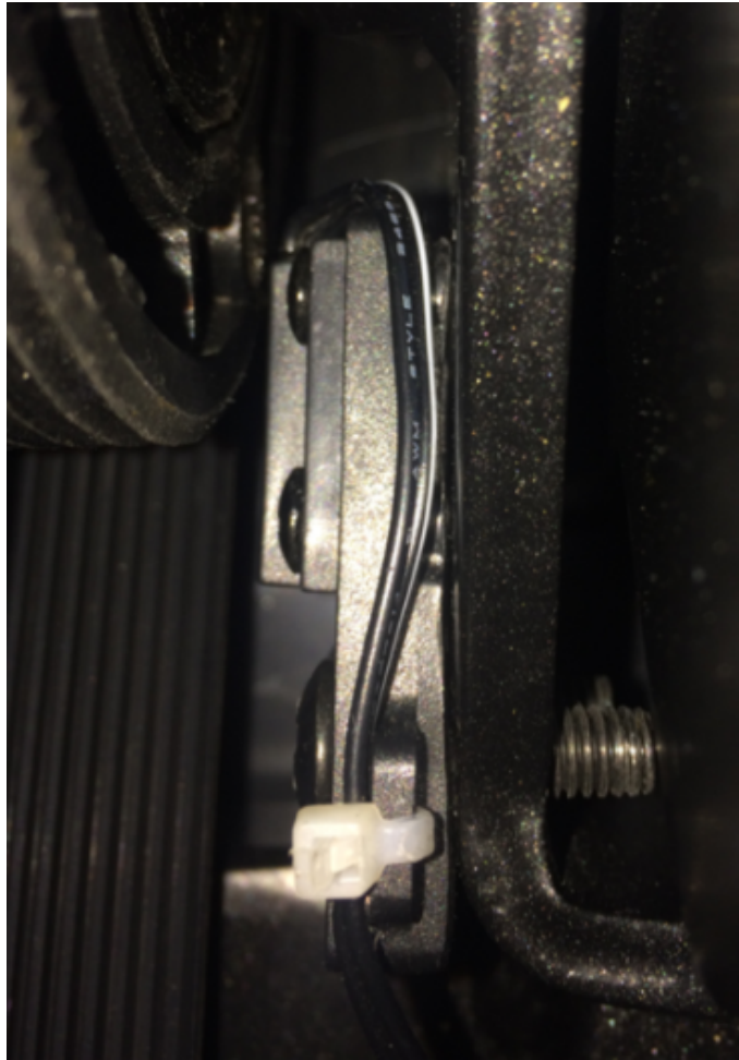
An example of a properly positioned speed sensor and wire.
