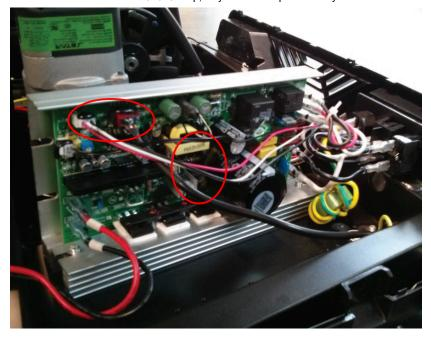
The position of lights on the MCB has changed several times during production. The most common location of lights are circled in red but they may be located elsewhere on the MCB if you have a different model MCB.
