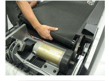
16. Using a 6mm hex wrench, attach the Front Roller to the Bracket.
