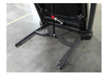
12. Using a 6mm hex wrench, remove both of the Adjustment Bolts from the Rear Roller.
