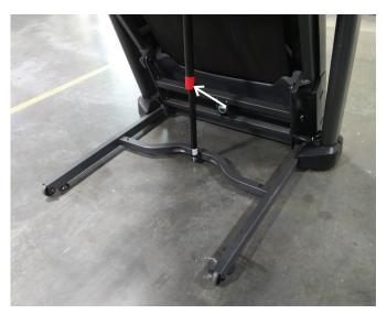
10. Using a #2 Phillips screwdriver, remove the 2 indicated screws (by arrow) that attach the Speed Sensor to the Frame near the Drive Pulley.
