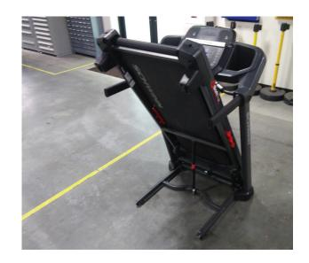
5. Using a #2 Phillips screwdriver remove the 2 indicated screws from the Motor Cover and remove it.
