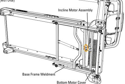
12. Using a #2 Phillips screwdriver, remove the 7 indicated screws from the Bottom Motor Cover.
