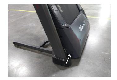
6. Make sure there is sufficient space to lower the walking deck.
