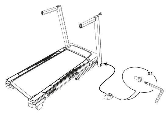
17. Connect the Cables and Attach the Console to Frame Assembly
