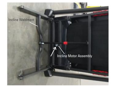
9. Using a 16mm and a 17mm wrench in the Motor Compartment, remove the hardware from the Incline Motor Assembly. Remove the Incline Motor Assembly noting how it extends from the Motor Compartment through to the Incline Weldment.
