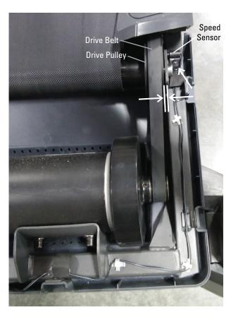
13. Using a 6mm hex wrench, remove the indicated screw from the Front Roller.
