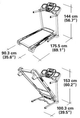
Select the area where you are going to set up and operate your machine. For safe operation, the location must be on a hard, level surface. Allow a minimum workout area of 190.3 cm x 376.2 cm (74.9" x 148.1"). Be sure that the workout space you are utilizing has adequate height clearance, taking into consideration the height of the user and the maximum incline of the machine.
