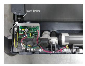
20. Using a 6mm hex wrench, remove the 2 indicated screws from the Deck
