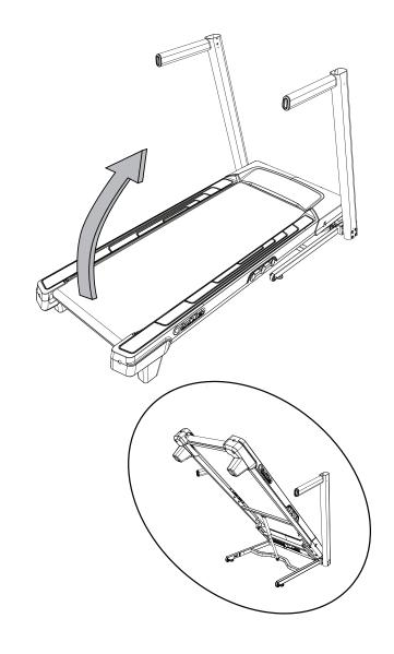
8. Using a 6mm hex wrench, remove the hardware that secures the Right Upright and slightly shift it away from the Frame Assembly. Carefully remove the I/O Cable from the old Right Upright, and dispose of the old Right Upright appropriately.
