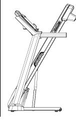
7. Make sure that the locking mechanism is engaged. Carefully pull back on the Walking Deck and make sure that it does not move. When you do this, keep clear of movement path in case the treadmill lock is not properly engaged.
