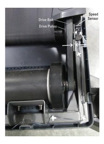
13. Using a 6mm hex wrench, remove the indicated screw from the Front Roller.
