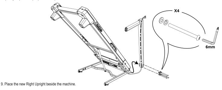
10. Connect the I/O Cable to the guide wire found at the lower part of the Right Upright. Gently route the I/O Cable through the new Right Upright.
