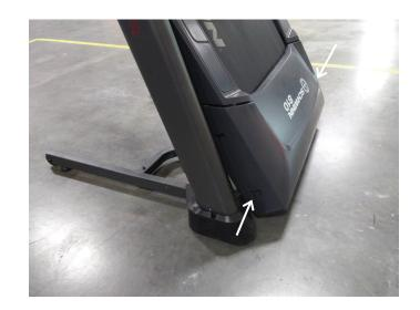
6. Remove the connectors for the Incline Motor Potentiometer and the Incline Motor from the Motor Control Board after noting their locations.
