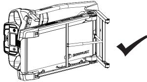
6. Using a 13mm wrench and a 6mm hex wrench, remove the indicated hardware (with ovals) from the Lift Shock Assembly.
