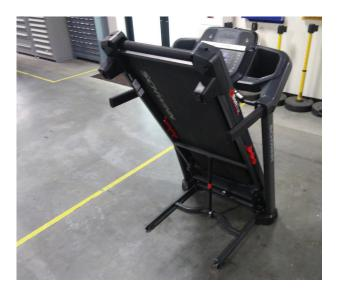
8. Using a #2 Phillips screwdriver remove the 2 indicated screws from the Motor Cover and remove it.
