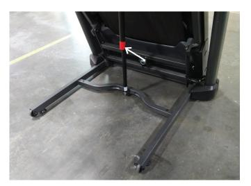
12. Be sure to observe the distance from the Speed Sensor to the Drive Pulley. This distance affects the effectiveness of the Speed Sensor, and can easily be shifted accidentally during replacement procedures.
