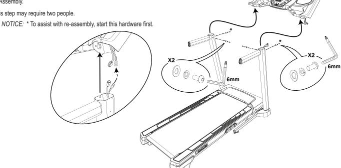
4. Re-install all parts that were removed in reverse order using the new Console Assembly.
