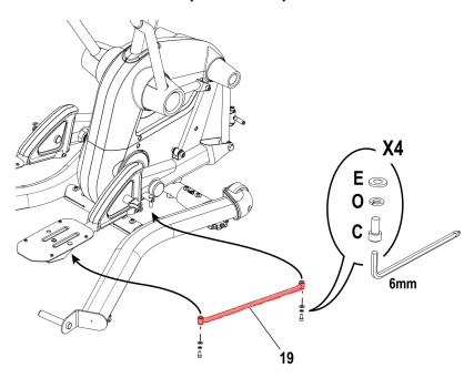
The right-side parallel link is highlighted in red. Tighten the hardware shown on both sides.
