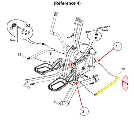
The right-side lateral link is highlighted in yellow. Tighten the hardware circled in red on both sides.
