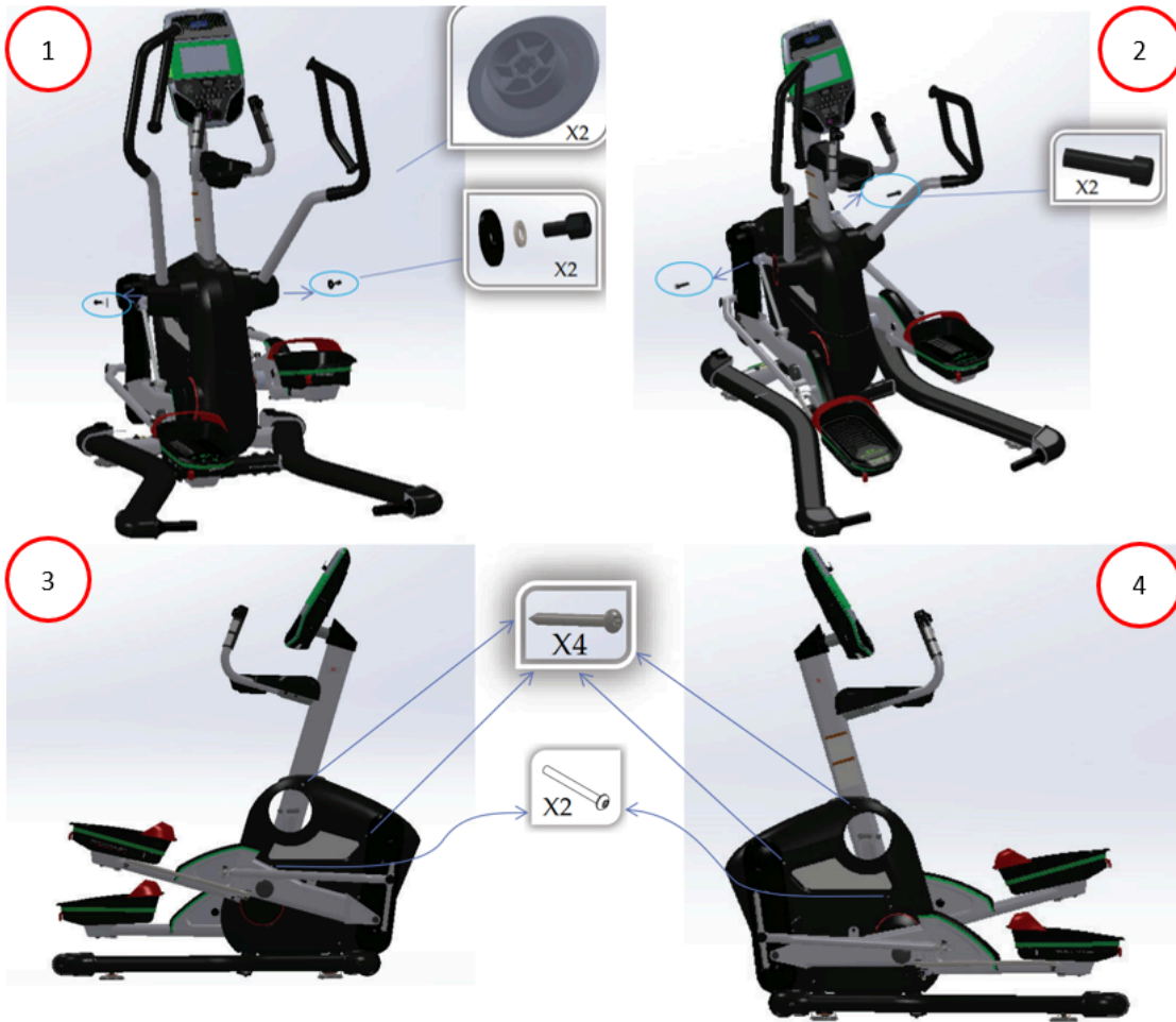
1-2: Remove the handlebars and set to the side. 3-4: Remove both upper shrouds and set to the side.
