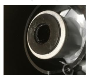
The handlebar inserts into the handlebar bushing, shown here.
