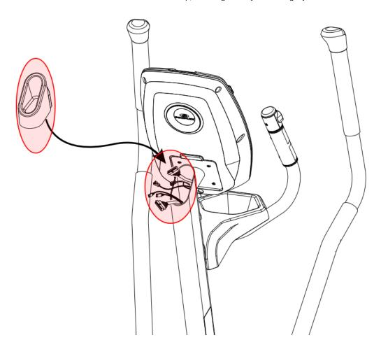
Remove the end cap, circled on the left, from the console mast and inspect the cables inside the console mast.
