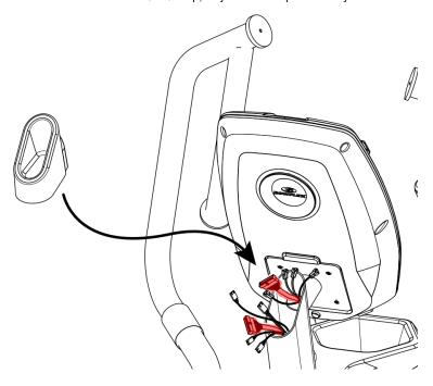
Remove the console mast cover and disconnect only the 8-pin cable (highlighted red).
