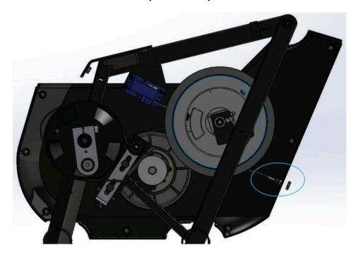
The power inlet pluq and power inlet wire are circled in blue on the right side of this image.
