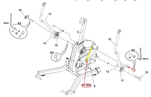
The right-side handlebar link is highlighted in yellow. Tighten the hardware circled in red on both sides.
