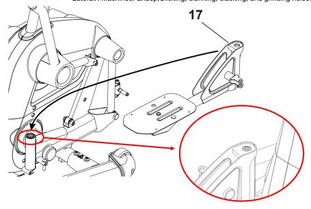
The top of the collared washer should be visible through the hole on the pedal arm.
