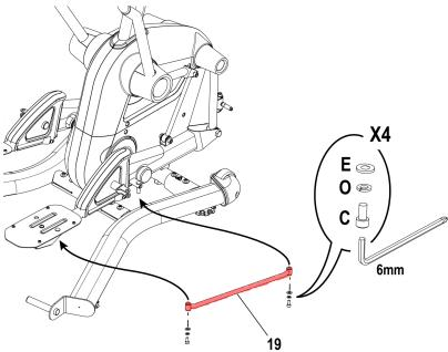
The right-side parallel link is highlighted in red. Tighten the hardware shown on both sides.
