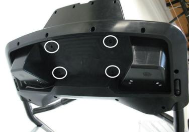
Remove the back of the console to secure the safety key receptacle inside the housing.
