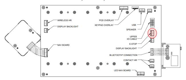
Inspect the wiring to the safety key receptacle and the connection at the console circuit board.
