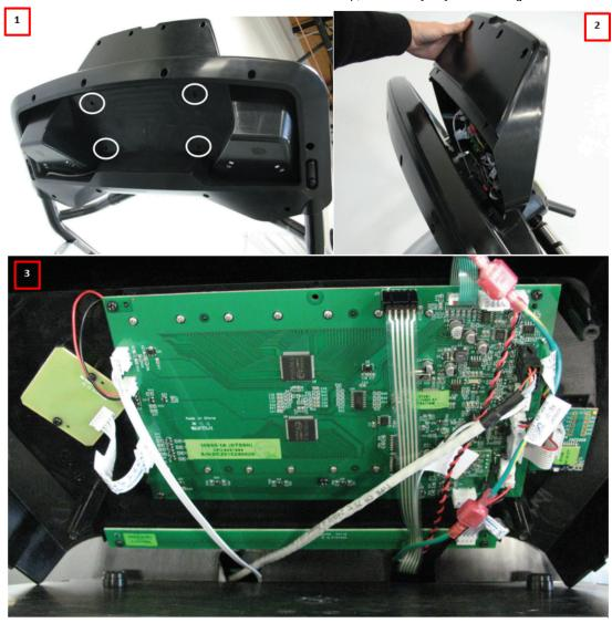
Remove the indicated screws (1) and tilt the console towards the buttons on the console main body (2) to expose the circuit board (3).
