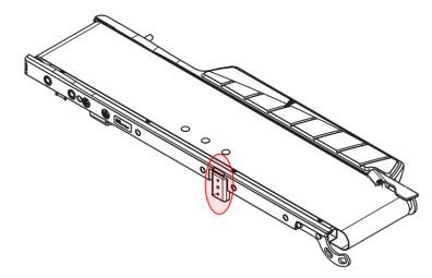
The friction block is circled in red - inspect for damage and check if it is loose or wobbly.
