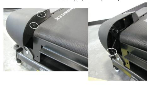
Remove the screws indicated and set the pivot cover to the side.
