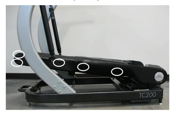
Remove the 5 screws from the left side cover and set the cover to the side to expose the motor and MCB.
