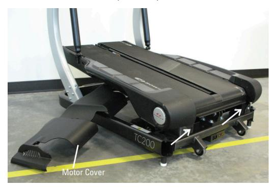
Remove the 2 screws indicated on the motor compartment cover, then remove the cover and set it off to the side.
