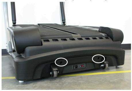
Remove the screws indicated on the rear cover and set the cover to the side.
