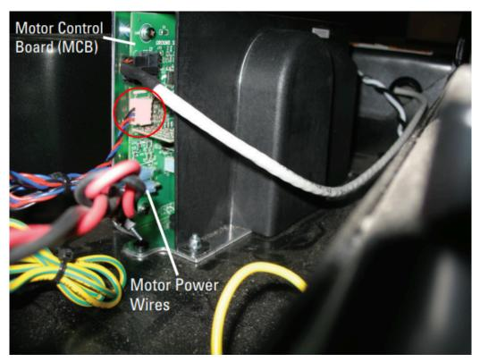
Inspect the bundle of red/black/blue wires for damage and make sure that the wires are firmly connected at the MCB.
