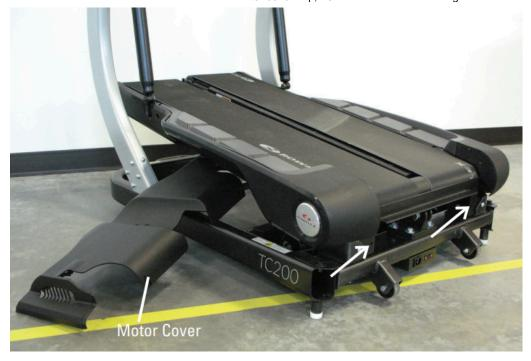
Remove the 2 screws indicated on the motor compartment cover, then remove the cover and set it off to the side.
