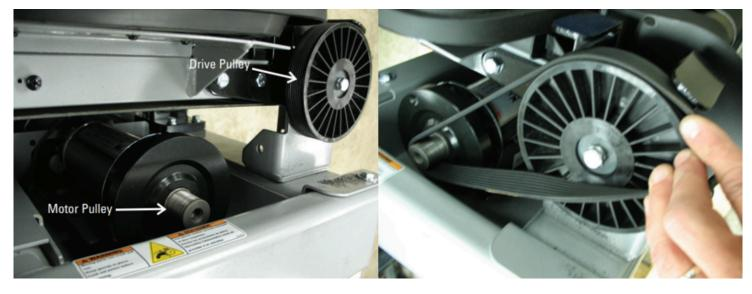
The drive belt should be tight across the drive and motor pulleys and free from damage, such as nicks, tears, or other excessive wear.
