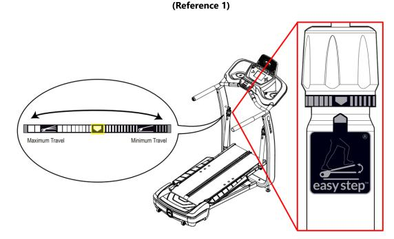
The EasyStep Shock adjustment dials are found on the hydraulic cylinders at the front of the machine. Adjust the dials until they are set to the center setting, shown highlighted in yellow in this image.
