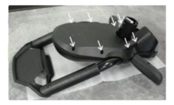
The white arrows indicate the location of the screws to remove in order to remove the console's rear shroud.
