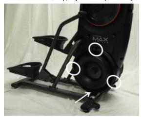
The white arrow indicates the location of the power plug wire inlet and bottom screw. The bottom screw can be loosened 3 turns rather that removing it entirely. The white circles indicate the locations of the screws to remove in order to remove the cover.
