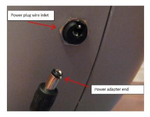
This image provides an example of damage to the power adapter end and the power plug wire inlet.
