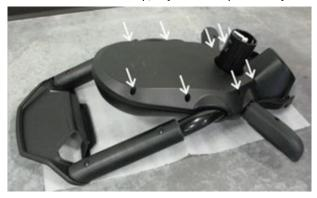
The image shows the rear side of the Max Trainer M7 console. The white arrows indicate which screws to remove in order to access the input/output cables.
