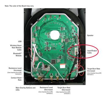
The board is shown with the location of the input/output cable circled in red on the right.
