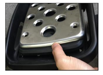
This image shows the four layers that the screw needs to be inserted through.
